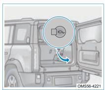
There is an electronic lock unlocking button on the luggage compartment right inner garnish. Manually unlock the button to unlock the cable.
