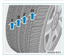
Check the tire tread for tread wear mark. When tread wear reaches its limit, tread will be in the same plane as the wear band. If such condition occurs, it indicates that performance and safety of tire seriously decrease, and replacement is necessary.
