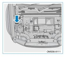
VIN is attached on the front of the front right shock absorber seat. Open the hood, VIN can be seen in the front of the front right shock absorber seat.
