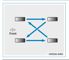
To equalize tire wear and extend tire service life, we recommends that four tires are rotated every 10,000 km (the best adjustment and rotation range is 5,000 - 7,000 km); the tire rotation cycle may vary according to driver's driving habits and road surface conditions.
