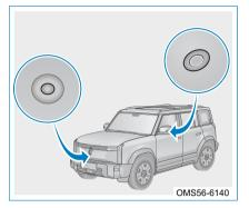
Installation position of front camera: Intake grille of front bumper.
