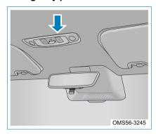
The emergency power-off switch is located on the driver's ceiling.
