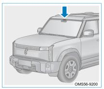
The microwave window is located on the inner side of the front windshield and at the right side to the back of the inside rear view mirror, where is for wireless RF signal transmission and installation of automotive electronic identification.
