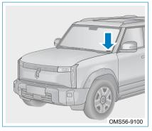
VIN is attached on the left side of the instrument panel near the A-pillar, and it can be seen through the front windshield.
