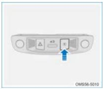
If you need to power off the vehicle forcibly in an emergency, long press the emergency power-off switch for 3 seconds or press the emergency power-off switch three times continuously within 3 seconds to power off the vehicle.
