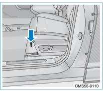
VIN is stamped on the seat beam under the front passenger seat. Fully move the front passenger seat back and lift the carpet to see it.
