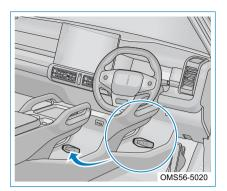
When smart key battery is low or signal is seriously interrupted, start and stop function will not work normally. In this case, start vehicle according to following steps:
