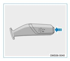
When the vehicle is stationary, depress brake pedal, when shift position is not in P, press the button on right side of column shift to switch to P directly and exit the corresponding R/N/D, the electric parking brake automatically turns on at the same time and "(P)" indicator on instrument cluster remains on.
