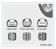
Incorrect tire inflation pressure will to excessive lead power consumption, shorten the tire service life and reduce the vehicle stability. Therefore, you should drive the vehicle with proper tire pressure (For provisions about the tire inflation pressure, please refer to the tire pressure label on driver side B pillar). When cold tire inflation pressure is specified than economic tire pressure is used, driving comfort will be reduced accordingly. Please adiust according to your needs.
