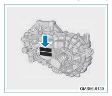
The front decelerator label is attached on the front decelerator housing.
