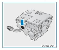
The rear drive motor label and steel seal number are printed on the rear drive motor housing.
