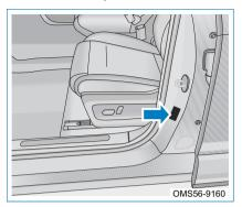
The vehicle name plate is located on the lower part of the front left door quarter outer panel door buckle.
