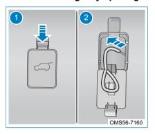
When the electronic inner door opening button fails to open the four-door, the emergency inner door opening pull ring can be used for emergency opening.
