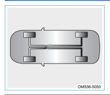
Brake system adopts X type dual circuit brake system. This system is a hydraulic system which has two independent sub systems. When one of the sub systems is not working, the other sub system can still implement the braking function.
